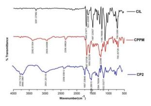
Fig. 2: FTIR spectral interpretation of cilnidipine-Lphenylalanine cocrystal and its components
