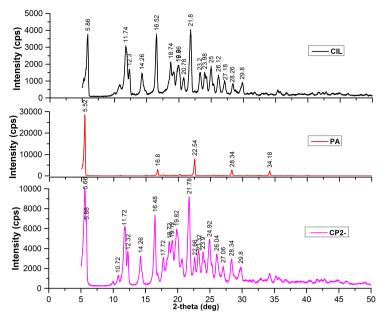
Fig. 4: PXRD pattern of cilnidipine (Cil), L-phenylalanine (PA) and cilnidipine-L-phenylalanine cocrystal (CP2)
