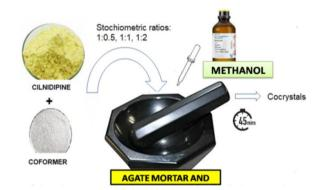
Fig. 1: Schematic representation of LAG for preparation of cilnidipine-L-phenylalanine cocrystals
