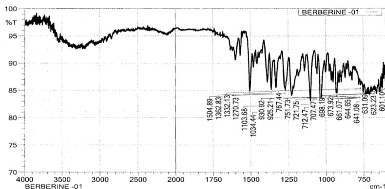
Fig. 2(b): FT-IR spectra of BBH
