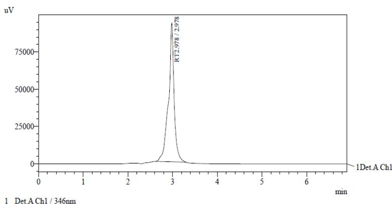
**Fig. 1: Chromatogram of BBH in potassium dihydrogen orthophosphate buffer (50 mmol) with a flow rate of 1.0 ml/min**
