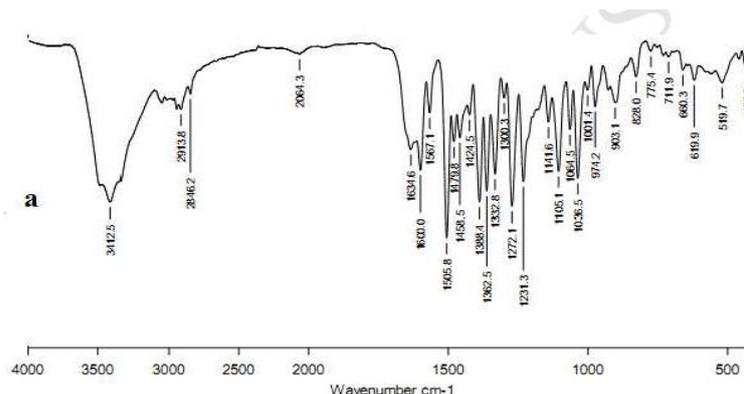
**Fig. 2 (a): FT-IR spectra of BBH (Reference) [23]**
