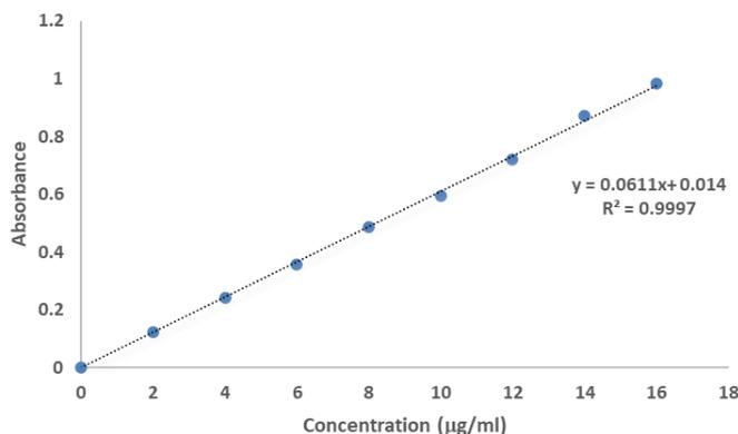
Fig. 1: Calibration curve of ESPO
