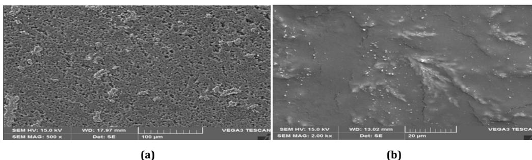
**Fig. 4: SEM images of a) Escitalopram oxalate placebo film(PVA) b) Optimized film formulation**
