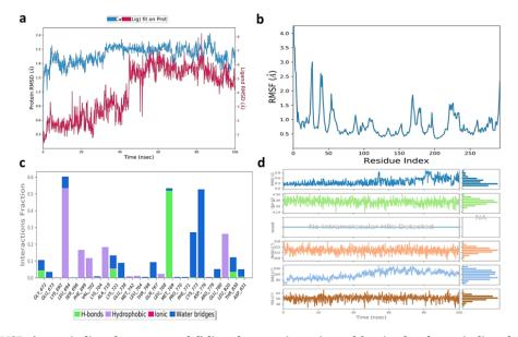
Fig. 3: a) RMSD, b) RMSF, c) protein-ligand contacts, and d) ligand properties estimated for simulated protein-ligand complex using 100 ns MD simulation
