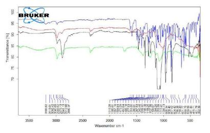
Fig. 7: FTIR spectrum of voriconazole pure drug and three polymers. Blue: voriconazole, red: PVA, black, PEO and green: HPMC
