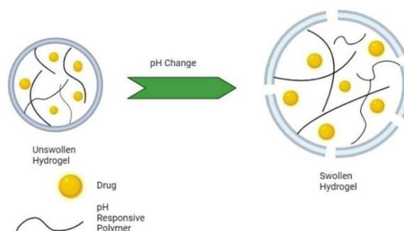
Fig. 3: Drug release by a change in pH resulting in swelling of the hydrogel [29, 37]
