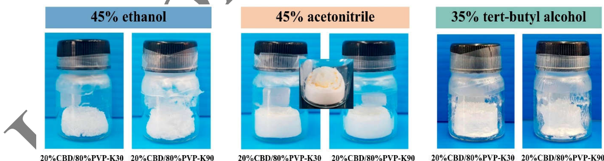
Fig. 4: Appearance of freeze-dried products prepared from binary solid dispersions containing 20% CBD and 80% polymer (PVP-K30 or PVP-K90) using different solvent systems: (a) 45% ethanol, (b) 45% acetonitrile, and (c) 35% tert-butyl alcohol. Corresponding formulations with PVP-K30 and PVP-K90 are shown for each solvent condition
