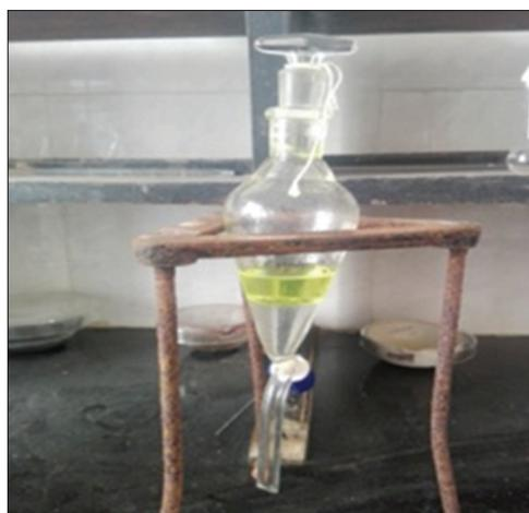
Fig. 6: Partition coefficient of *Haridra* extract by n-octanol and water media. (50:50)
