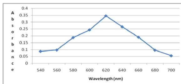
Fig. 2: Absorption spectrum of Chloramphenicol with MBTH/FeCl<sub>3</sub>
