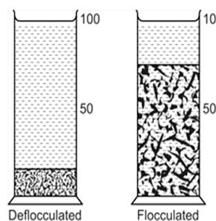
Fig. 1: Schematic representation of deflocculated and flocculated suspension
