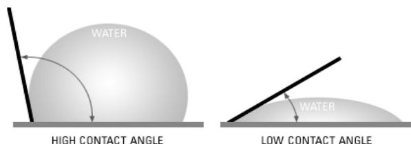
**Fig. 6: Schematic representation of water drops creating an angle on the solid surface**
