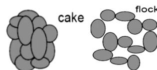
Fig. 2: Schematic representations of cake and flock formed in deflocculated and flocculated suspension respectively
