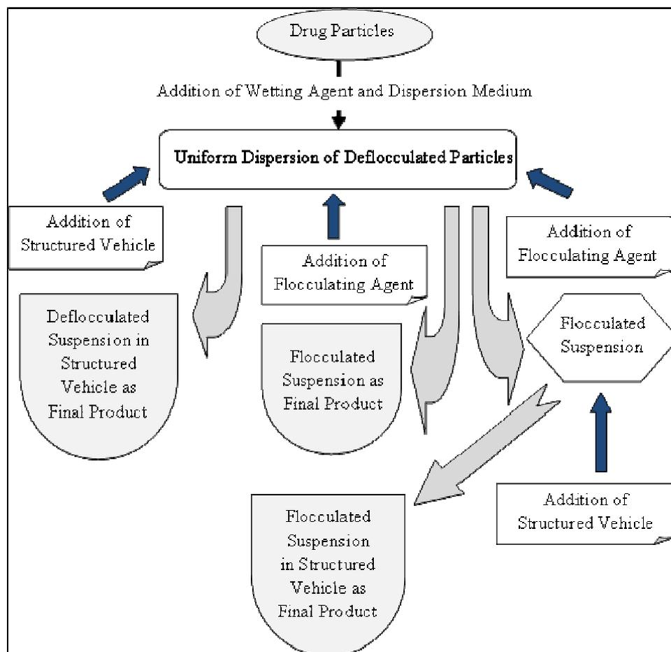
Fig. 3: Flow chart focusing the approaches for formulation of suspension
