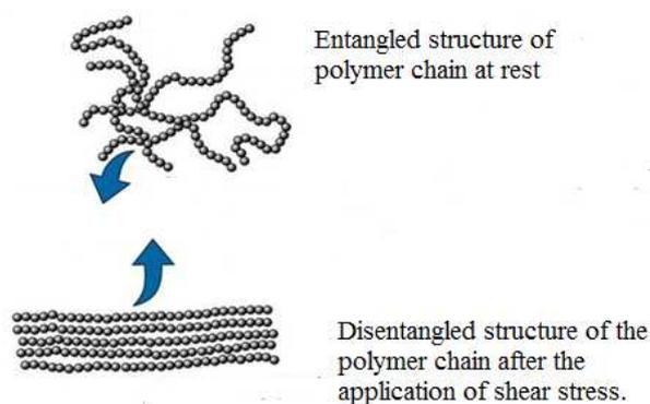
**Fig. 7: Polymer chain orientation before and after the application of shear stress**
