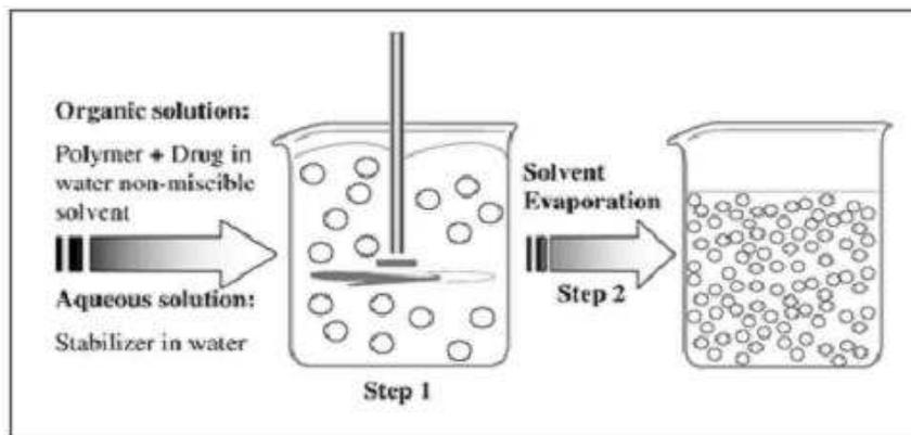
Fig. 3: Schematic representation of the solvent evaporation technique
