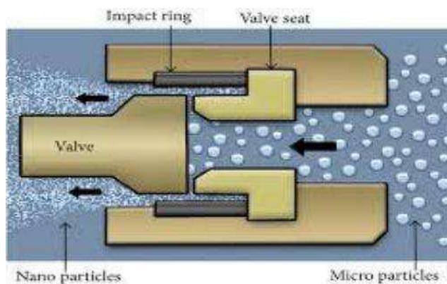
**Fig. 1: Schematic cartoon of the high-pressure homogenization process**
