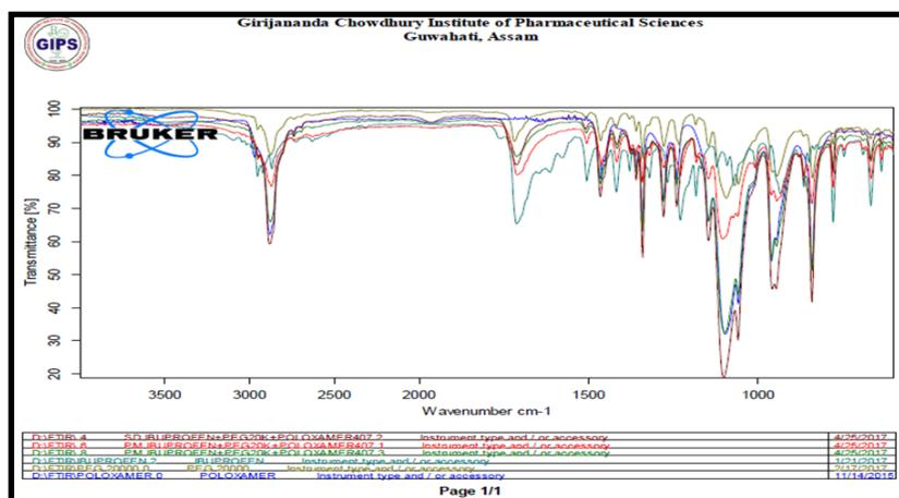
Fig. 4: IR spectra of ibuprofen, PEG 20000, poloxamer 407 and solid dispersions SDF7, SDF8, SDF9
