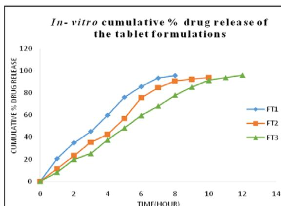
Fig. 8: In vitro cumulative % drug release of the tablet formulations
