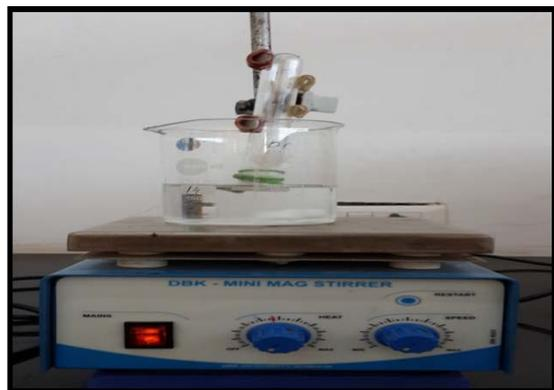
Fig. 3: Laboratory designed diffusion cell
