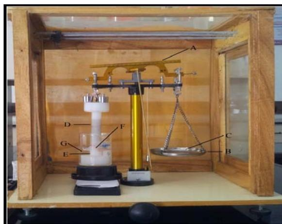
Fig. 2: Modified balance for mucoadhesive study, A: Modified balance, B: Weighing pan, C: Weight D: Gel, E: Nasal mucosa F: polypropylene cylinder
