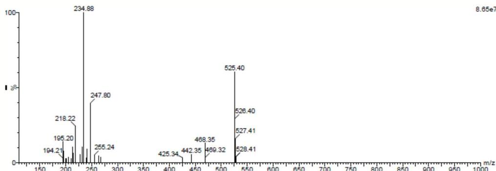
Fig. 5: Mass spectrum of dimer impurity
