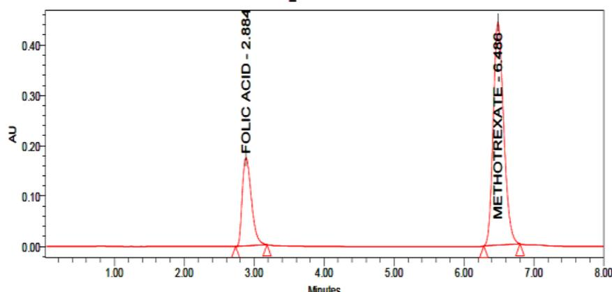
Fig. 26: Typical chromatogram of methotrexate and folic acid
