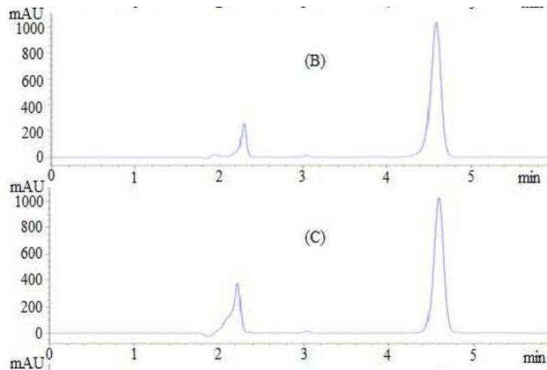
Fig. 33: Chromatogram of oxidative degradation of phenytoin (b), and base degradation (c)
