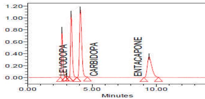
Fig. 13: Chromatogram of heat degradation of levodopa, carbidopa, and entacapone
