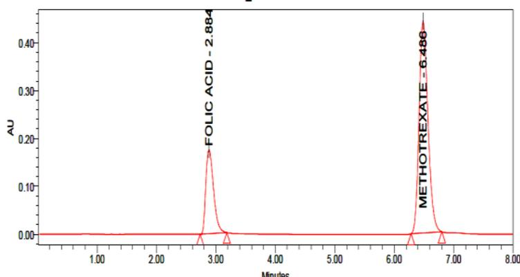
Fig. 19: Typical chromatogram of methotrexate and folic acid
