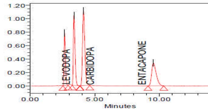
Fig. 14: Chromatogram of alkaline degradation of levodopa, carbidopa, and entacapone
