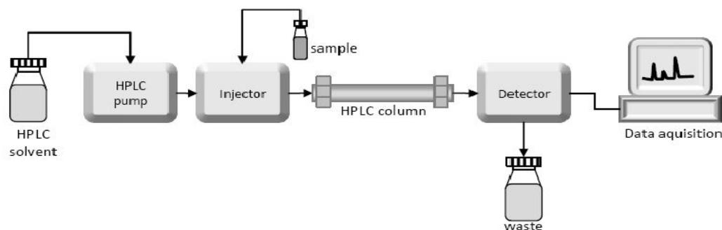
Fig. 1: Instrumentation of HPLC
