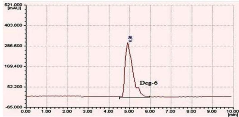
Fig. 31: Chromatogram of phenobarbitone after dry heat degradation
