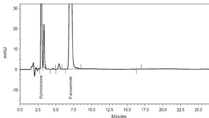
**Fig. 23: Chromatogram of alkali degradation of spironolactone and furosemide**
