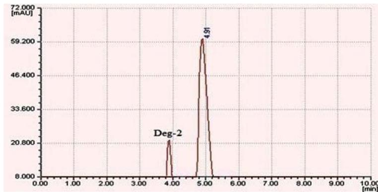
Fig. 29: Chromatogram of phenobarbitone after alkali hydrolysis
