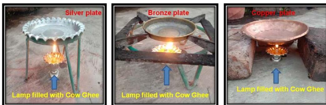
Fig. 1: Preparation of carbon soot by using different metal plates spreaded with *Aloe vera* mucilage
