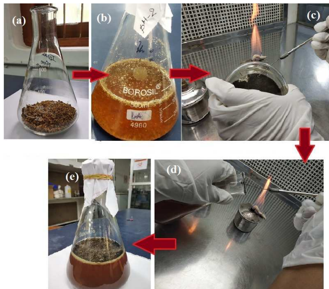
Fig. 4: (a,b)-Pomegranate peel supplemented basal fermentation media; (c,d)-inoculation of fermentation broth media; (e) Mycelial Growth of A. niger in fermentation media
