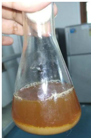
Fig. 5: Precipitation of calcium sulphate leaving calcium citrate in the solution
