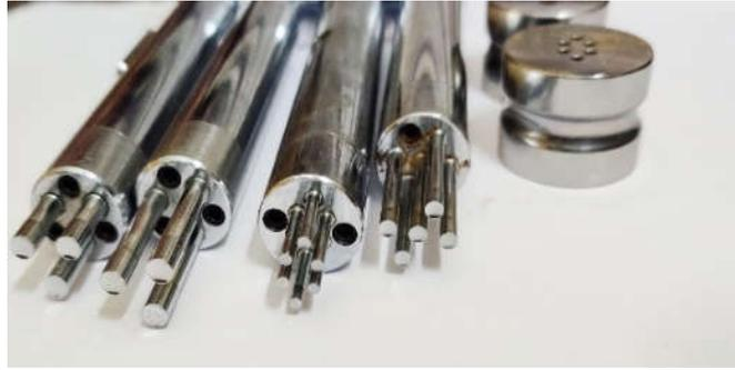
Fig. 2: It shows tip sizes of the multi tip punches/compression
