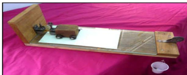
Fig. 1: Laboratory designed tensile strength tester
