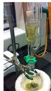
Fig. 1: Soxhlet apparatus
