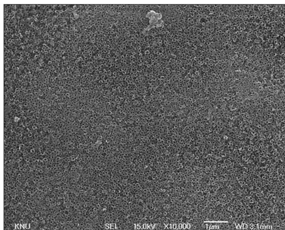
Fig. 1: Scanning electron microscopy of titanium oxide nanotube surface
