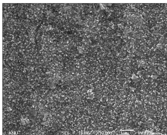
Fig. 3: Scanning electron microscopy of Cu-HA surface
