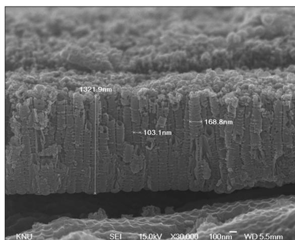
Fig. 2: Scanning electron microscopy of the cross-section of titanium oxide nanotube surface
