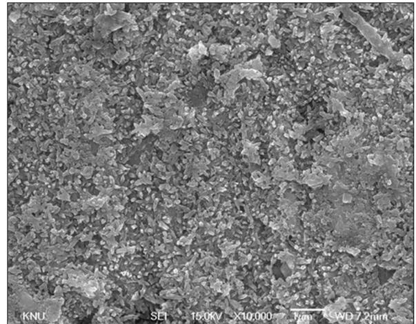
Fig. 4: Scanning electron microscopy of Zn-HA surface
