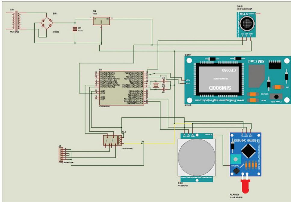
Fig. 2: Circuit diagram of the proposed smart home system
