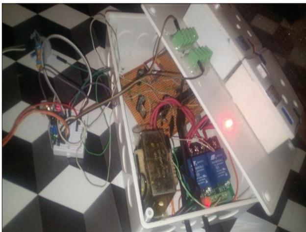
Fig. 5: Interfaced system with relay
