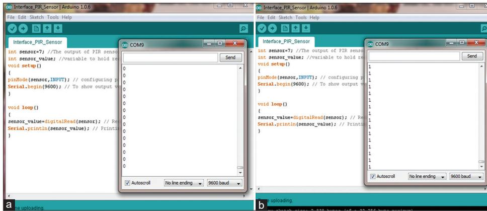
Fig. 4: (a) Simulation of PIR sensor from Arduino IDE when there is no motion inside the range (b) Simulation of PIR sensor from Arduino IDE when motion detected
