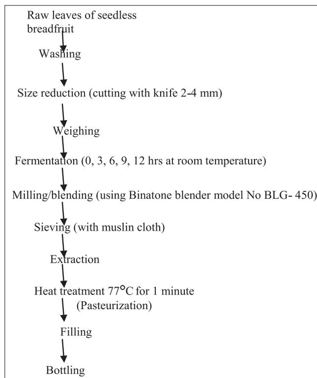
**Fig. 1: Flow diagram of processing of *Artocarpus communis* leaves into leaf extract**
