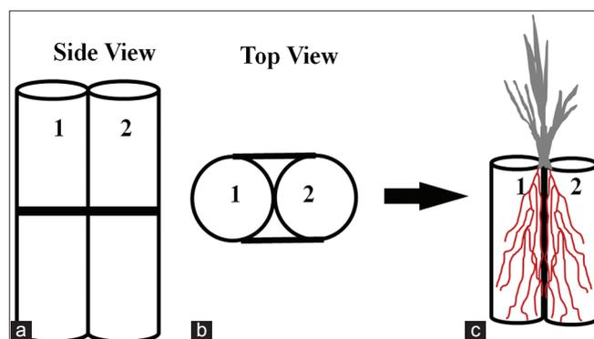
Fig. 1: Schematic representation of split-root setup. (a) Side view and, (b) Top view of the polyvinyl chloride pipes joined together. (c) Seedling transferred in split-root setup
