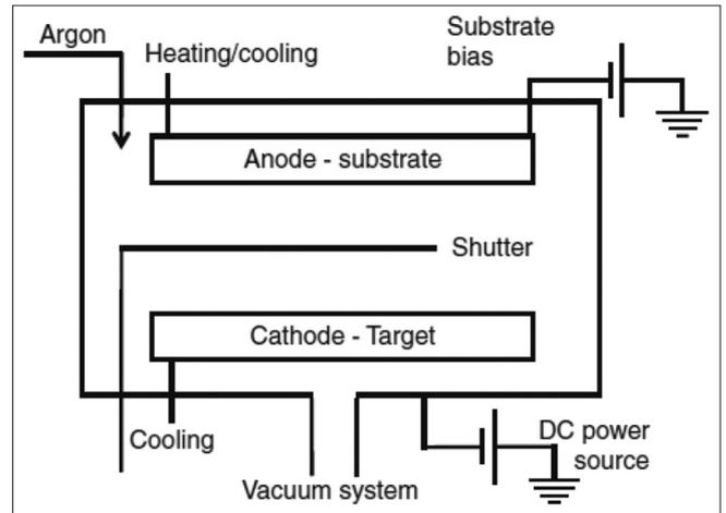
Fig. 3: A schematic of direct current sputtering chamber with the main and important factors that effect on the process [9]
