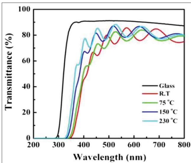
Fig. 5: The relationship between transmittance spectra of ultraviolet visible between 200 and 800 nm of Ga-doped ZnO nanofilms with different substrate temperature (25, 75, 150, and 230°C) [12]
