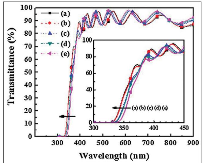
Fig. 6: Transmittance spectra of ultraviolet visible radiation for wavelength (200–900) nm of Al-Y co doped ZnO nano-thin films at different range of direct current sputtering pressure (5, 7, 11, and 13) mTorr [13]
