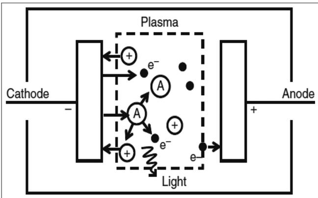
Fig. 1: A smile schematic of the plasma formation principle between cathode and anode [9]
