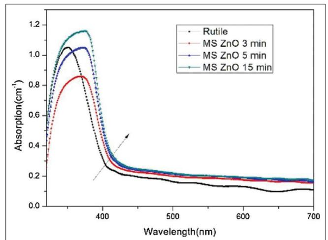
Fig. 4: The relationship between ultraviolet visible absorption and sputtering times (3–15) min, for wavelength range between 200 and 700 nm [10]
