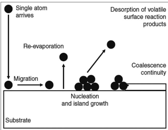
Fig. 2: A schematic of the main stages to format nano-films by direct current sputtering [9]
