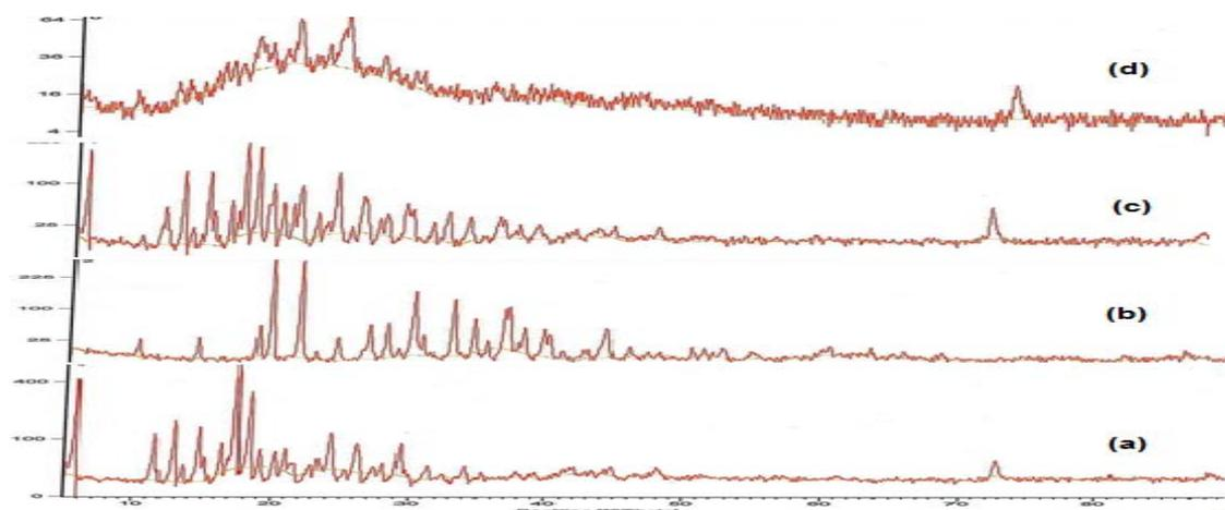
Fig. 4: X-ray spectra of CRV-tartaric acid systems, a) CRV alone, b) Pure tartaric acid, c) CRV-tartaric acid PM, d) CRV-tartaric acid SD
