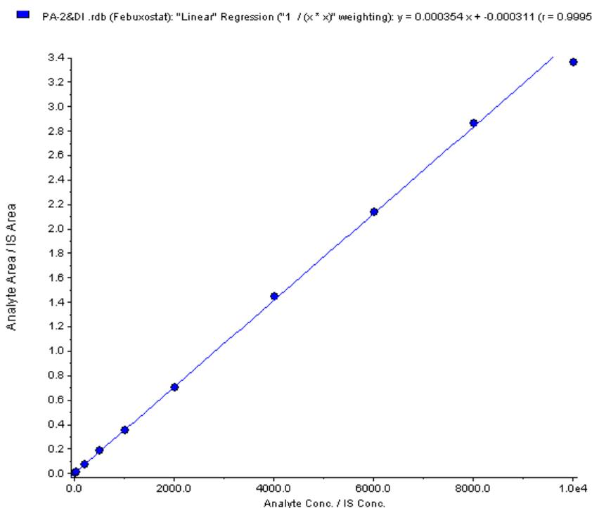
Fig. 4: Calibration curve for regression analysis of FBS
