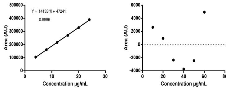
Fig. 7: Linear regression and residual plot for SIM
