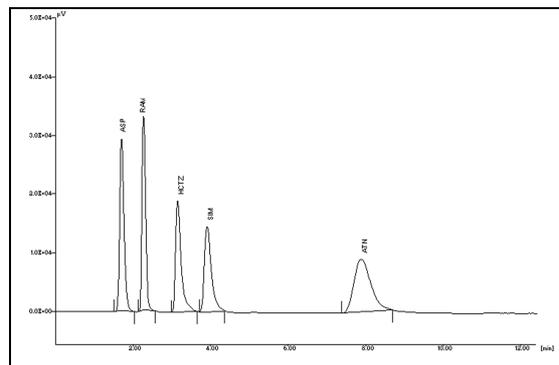
Fig.3: Chromatogram of ASP, RAM, HCTZ, SIM and ATN
