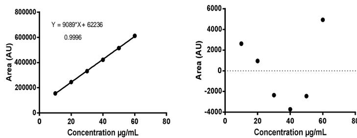
Fig. 8: Linear regression and residual plot for ATN
