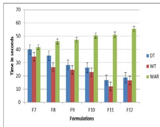
Fig. 12: Evaluations for disintegration time, wetting time, and water absorption ratio representation in column chart from formulations F7-F12
