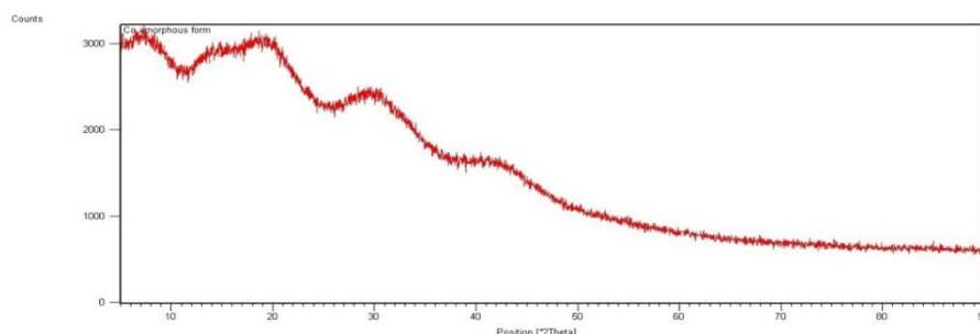
Fig. 10: X-ray powder diffractometer of co-amorphous AML-ATR
