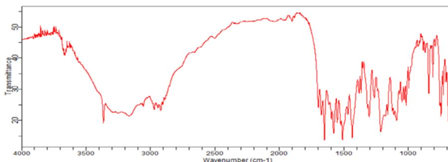
**Fig. 4: FTIR spectra of physical mixture of AML and ATR**
