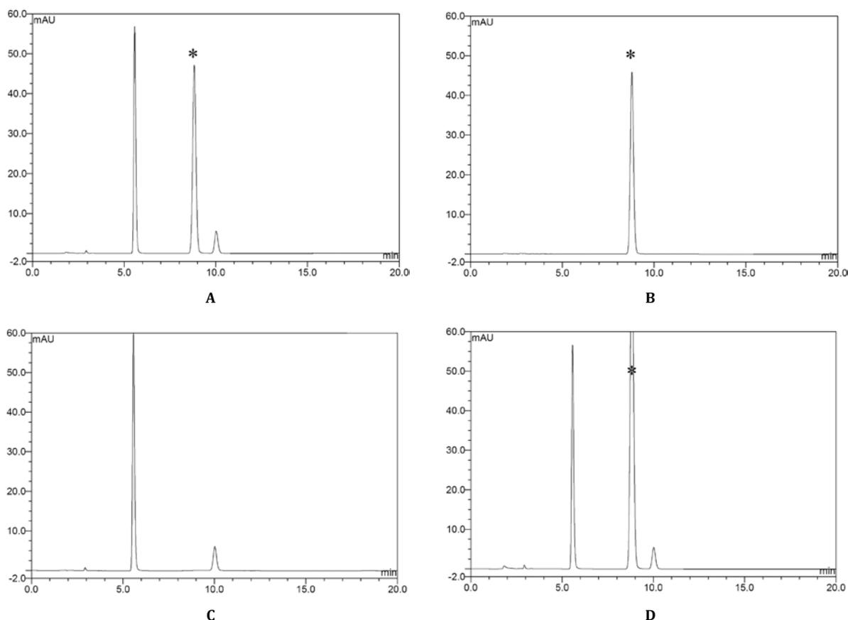
Fig. 2: Chromatographic separation of (A) extemporaneous sildenafil suspension, (B) sildenafil standard, (C) vehicle, and (D) standard-spiked extemporaneous suspension. \* indicated sildenafil peak.
