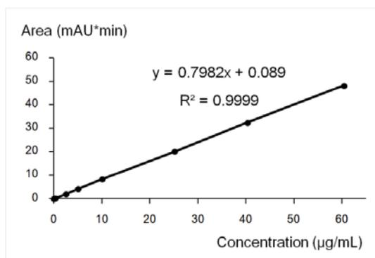
**Fig. 4: Calibration curve of sildenafil standard over a concentration range of 0.01 - 60.00 µg/mL.**
