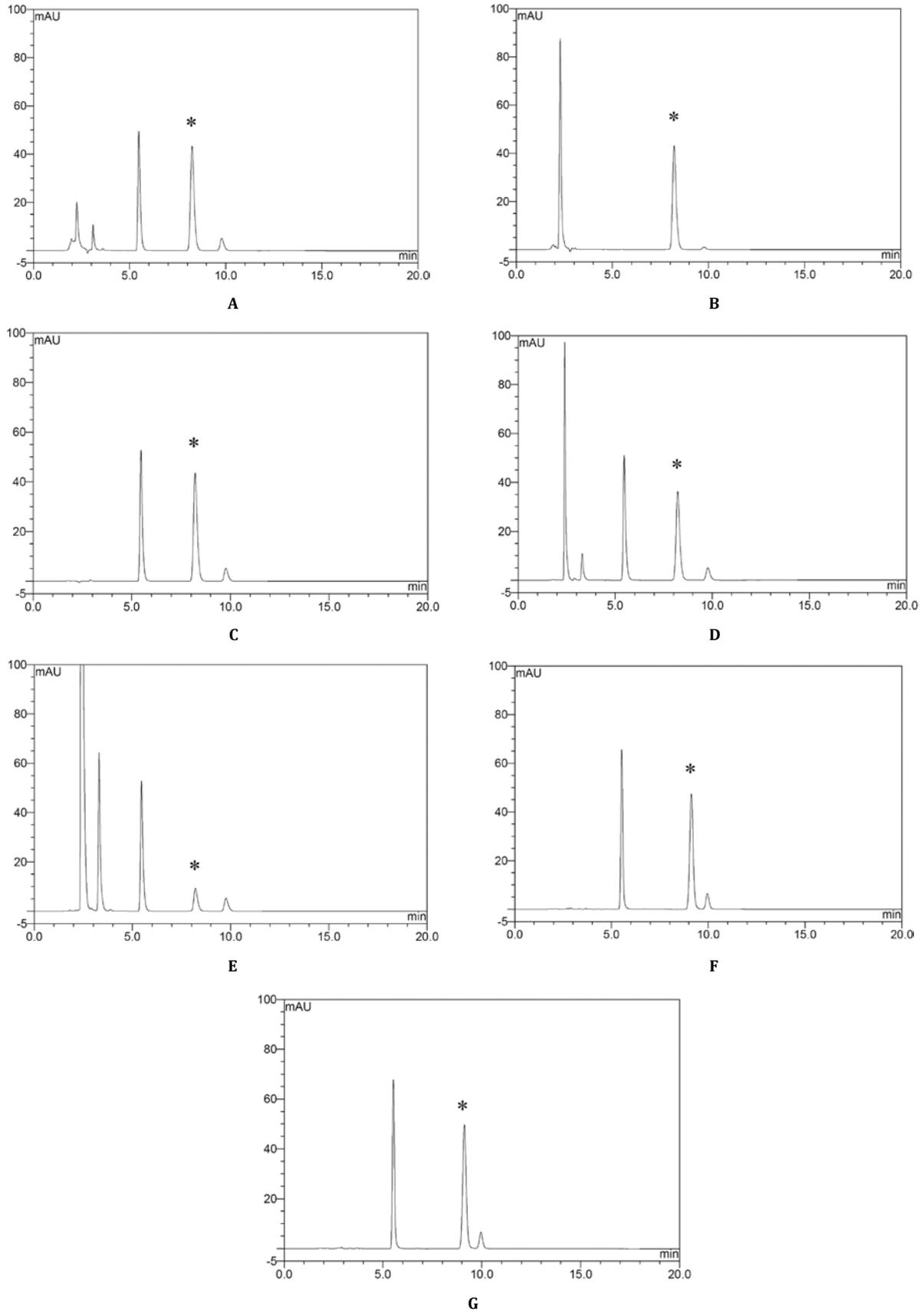
**Fig. 3:** Forced degradation studies of extemporaneous sildenafil suspension. (A) acid hydrolysis with 0.1 N HCl, (B) basic hydrolysis with 0.1 N NaOH, (C) neutral hydrolysis, (D and E) oxidation with 0.1% and 1.0% H<sub>2</sub>O<sub>2</sub>, respectively, (F) dry heat at 80°C, and (G) exposure to fluorescent lamp. \* indicated sildenafil peak.
