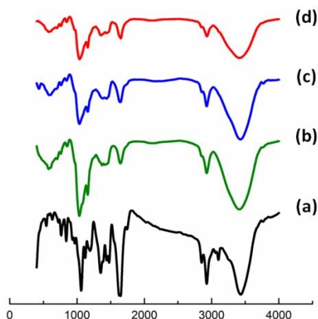
Fig. 7: FTIR spectrum of KH(a), MβCD(b), physical mixture (PM)(c) and freeze drying (FD)(d)
