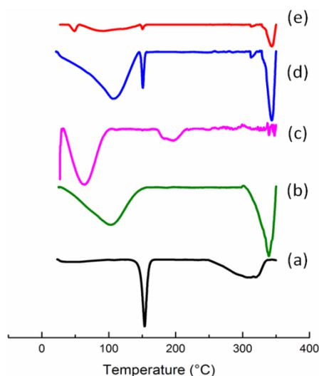
Fig. 4: DSC thermograms of KH(a), M $\beta$ CD(b), HPMC(c), physical mixture (d) and freeze drying (e)
