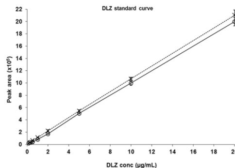
Fig. 2: Mean calibration curves for the determination of DLZ in water (x) and in human plasma (o) by HPLC using UV detector. (data are means  $\pm$  S. D., n = 6).
