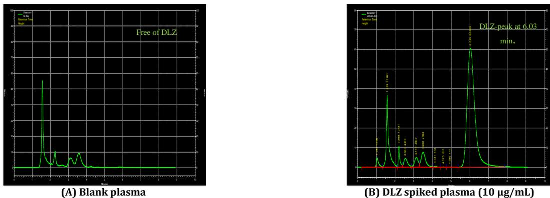
Fig. 1: Chromatograms of DLZ obtained from (A) plasma free of DLZ and (B) plasma spiked with 10  $\mu$ g/ml DLZ.
