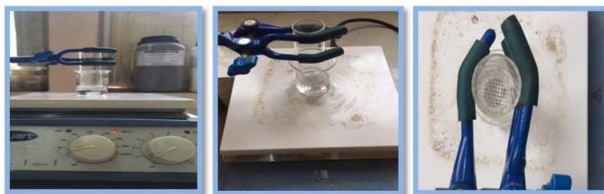
Fig. 2: Modified disintegration test apparatus used to determine the disintegration time of the prepared ODTs of zolmitriptan
