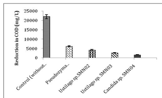
**Fig. 6: Reduction in COD (mg/L) of pharmaceutical wastewater after treatment with four yeast isolates. Data represents mean of triplicates with standard deviation of <5%**
