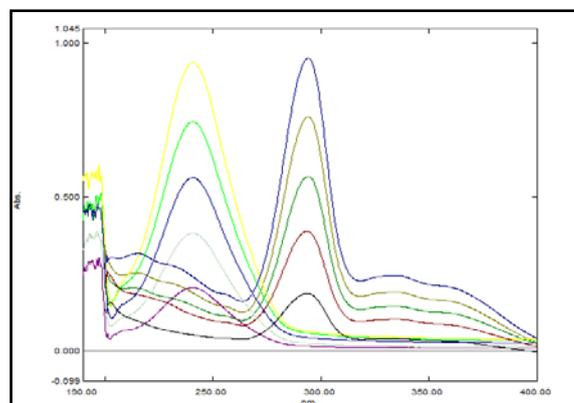
Fig. 3: Zero order Overlay spectra of Moxifloxacin HCl and Difluprednate.
