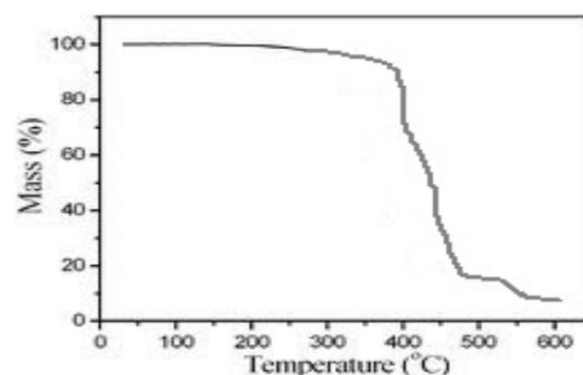
Fig. 2: It shows TGA curve of THQSA resin
