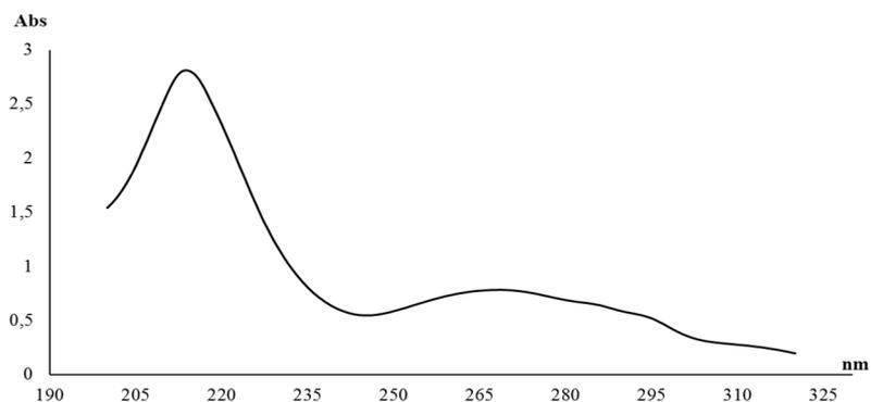
Fig. 3: UV absorption spectrum of VLB sulfate 40 µg/ml aqueous solution
