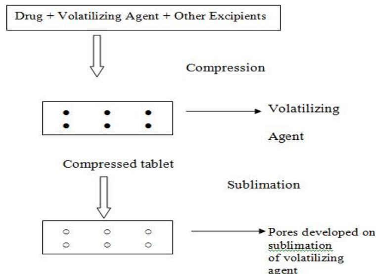
Fig. 2: Schematic Diagram of Sublimation Technique for Preparation of FDT [18]
