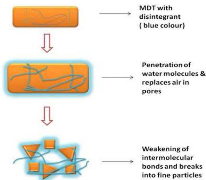
Fig. 1: Wicking mechanism. [26]
