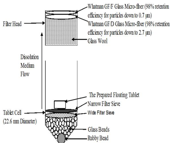
**Fig. 1: Dissolution cell design used for the prepared floating tablets: laminar flow with free tablet position (glass beads filling the entry cone).**
