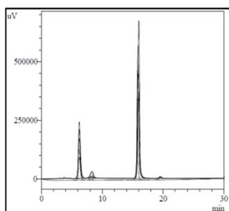
Fig. 6: Overlay Chromatogram for Linearity of HCTZ, OLM, HCTZ-IMP, OLM-IMP.
