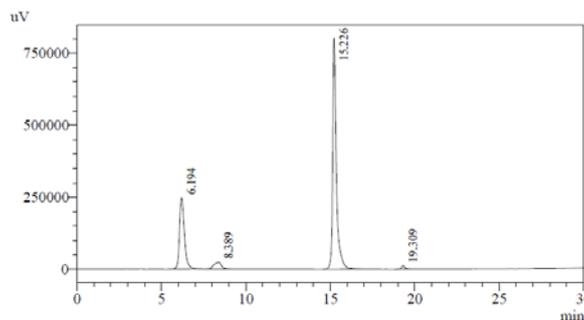
Fig. 5: Chromatogram of Mixture of HCTZ, HCTZ-IMP, OLM & OLM-IMP (125, 1.4, 200 & 2 µg/mL in ACN:Water-50:50 respectively)
