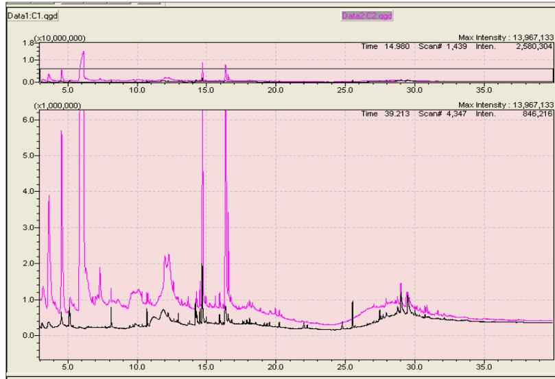
Fig. 14: An overlap chromatogram of GC of *in vitro* regenerated (hardened) and nature grown roots, C1 (Black) = *in vitro* regenerated root, C2 (Pink) = nature grown root
