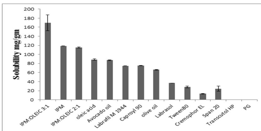
Fig. 1: Solubility of Co Q<sub>10</sub> in different oils, surfactants, and co-surfactants, IPM: isopropyl myristate, PG: Propylene glycol, mean±SD (n=3)
