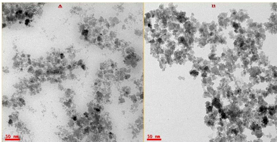
**Fig. 1: Characterization of TNP 20 and ZNP 20 particles by transmission electron microscopy (TEM). A-B: A. TNP 20; B. ZNP 20; all dispersions contained nanosized particles; however the particles were mostly dispersed as agglomerates or aggregates**
