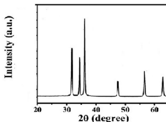
**Fig. 3: X-ray diffraction spectrum of ZNP 20**
