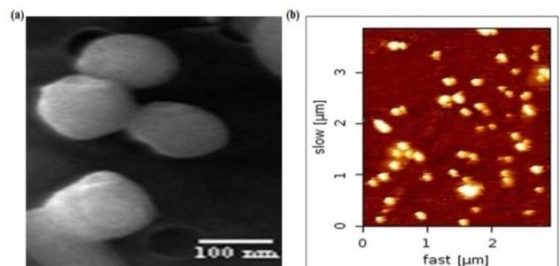
**Fig. 2:** (a) Scanning electron micrograph of (CUR+RAPA) loaded micelles (bar = 100 nm), (b) Atomic Force microscopy (AFM) images of (CUR+RAPA) loaded micelles.
