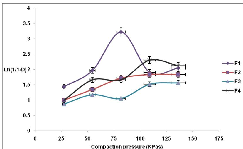
Fig. 2: Heckel plots of compacts of the different powder samples
