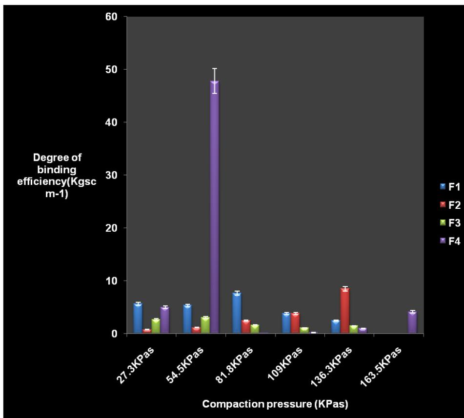
Fig. 3: Plot showing binding efficiency of compacts at different compaction pressures, three tablets were randomly selected and used for the determination for each batch at the respective pressure
