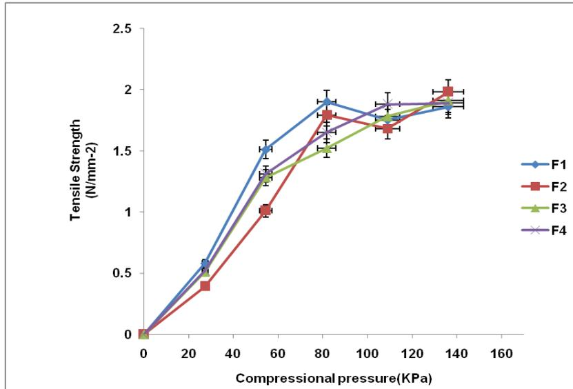
Fig. 4: Tensile strength–compressional pressure relationship, 3 tablets were used for the determination at the respective pressures
