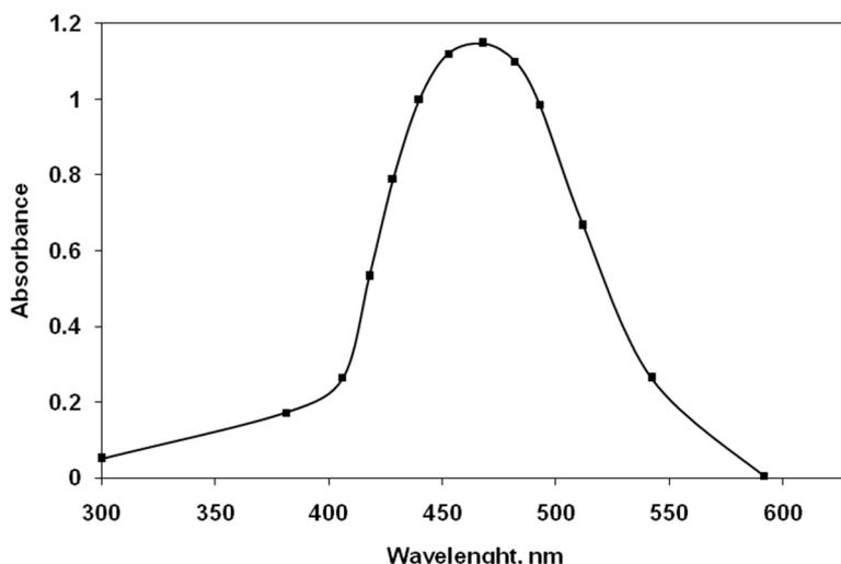
Fig. 2: Absorption spectra of 24  $\mu$ g/ml OXB with ECR dye complex extracted in dichloromethane
