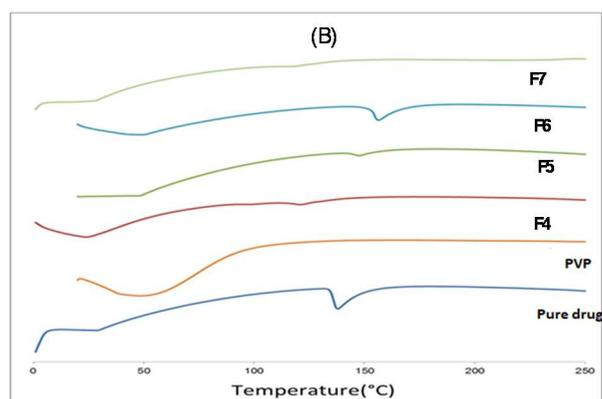
**Fig. 1: Examples of DSC traces of pure indomethacin, polyethylene glycol 6000 (PEG 6000), hydroxypropyl methyl cellulose E5 (HPMC), polyvinylpyrrolidone (PVP) and different formulations. For detailed formulations refer to table 1**
