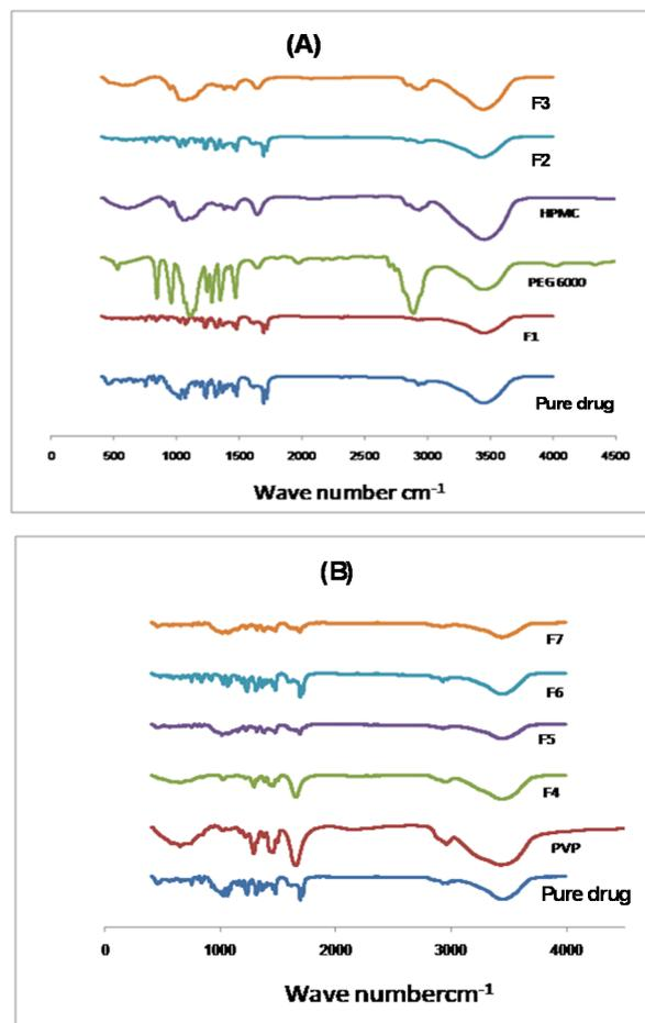
Fig. 3: FTIR spectra of unprocessed indomethacin and different formulations together with pure polyethylene glycol (PEG 6000), hydroxypropyl methyl cellulose (HPMC), and polyvinylpyrrolidone (PVP) together. For detailed formulations refer to table 1
