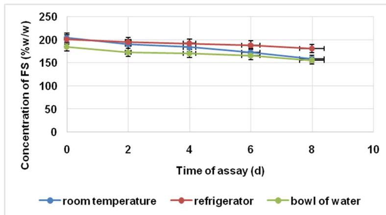
Fig. 1: Rates of degradation of flucloxacillin sodium (FS) in suspensions reconstituted with bottled water under the various storage conditions
