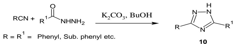
Scheme 4: An efficient base-catalyzed synthesis of 3, 5-disubstituted-1, 2, 4-triazoles
