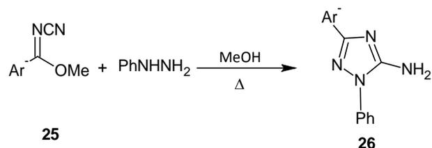
Scheme 10: Synthesis of 1,2,4-triazole derivatives via one-pot synthesis
