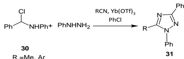
**Scheme 12: Ytterbium (III) triflate catalyzed synthesis of 1,2,4-triazoles**
