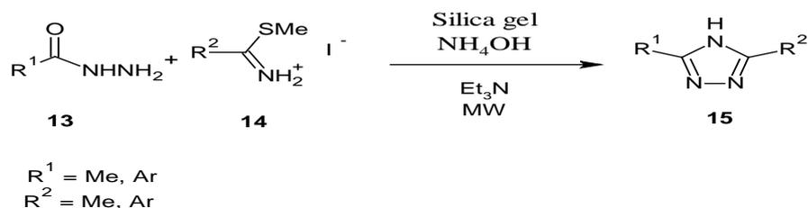
Scheme 6: Synthesis of 1, 2, 4-triazoles using silica gel
