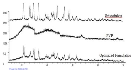
**Fig. 4: XRPD of griseofulvin, PVP, and optimized solid dispersion formulation**
